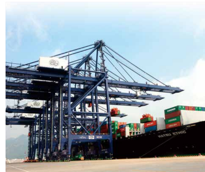
双 40 英尺箱岸边集装箱起重机 Quayside Container Crane for Double 40-Foot Containers
